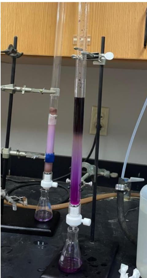
**Figure 7:** Sephadex LH-20 and G-50 Column Chromatography set up
