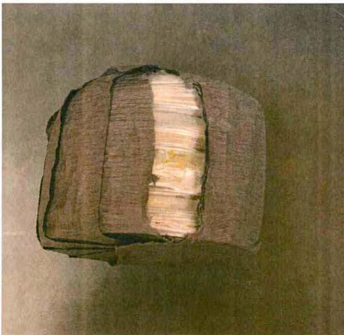
Figure 9: Plates wrapped in crepe streamers with a slit cut onto the light side of the plate
