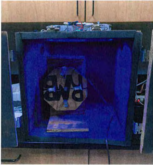
Figure 6: Blue light (460nm) incubator and clinostat
