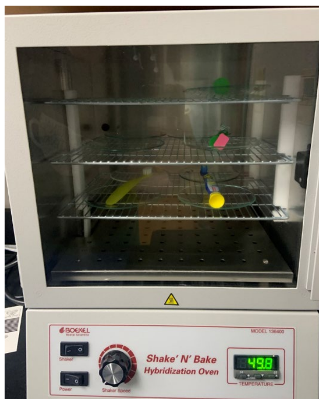
Figure 6: Shake'N'Bake Hybridization Oven from Boekel Scientific. Used to generate shipment environment.
