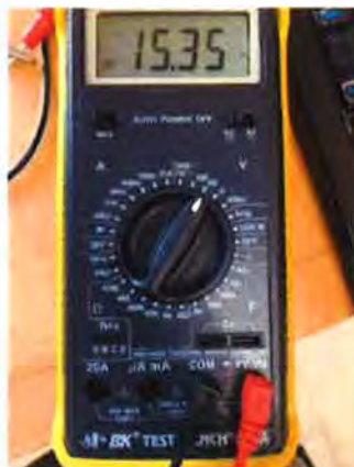
Make sure the red and black cords are plugged into voltmeter 1 as shown.
