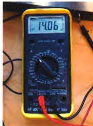
Make sure the red and black cords are plugged into voltmeter 2 as shown.
