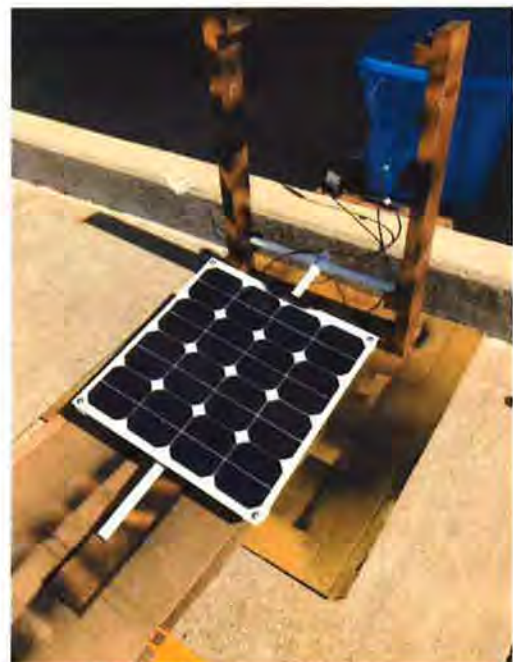
Figure 8: The solar panel set to the lowest of 3 settings on the stand is pointed toward the summer sun.
