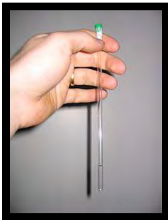
FIGURE 22: The photo above is of a glass tube used for ^1\text{H} -NMR.
