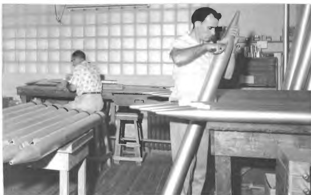
One of the flue voicing rooms. Pipes are shown in the process of preparation and voicing.
