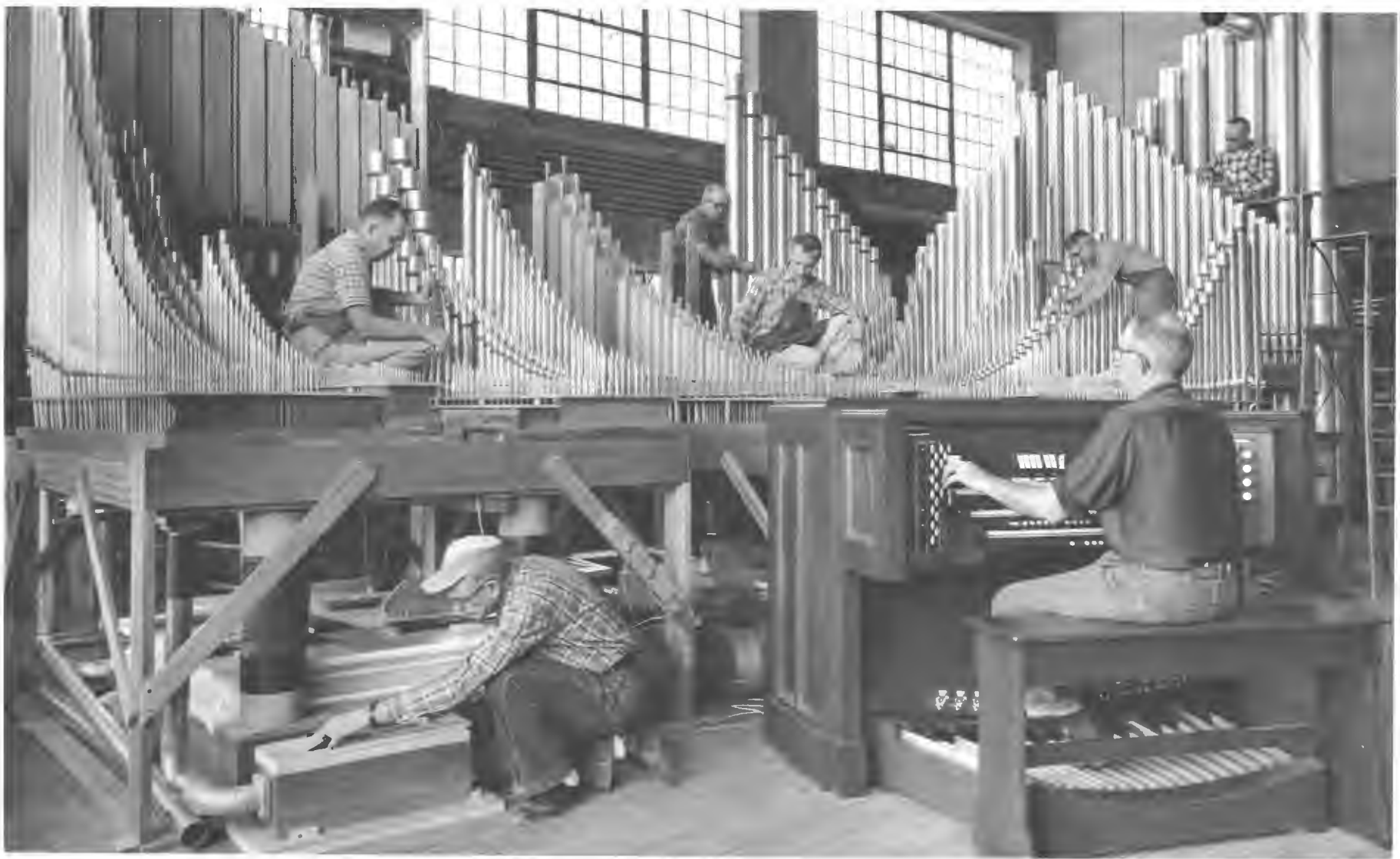
A view of the erecting room. The instrument shown is assembled for final testing before shipment to the site of installation.
