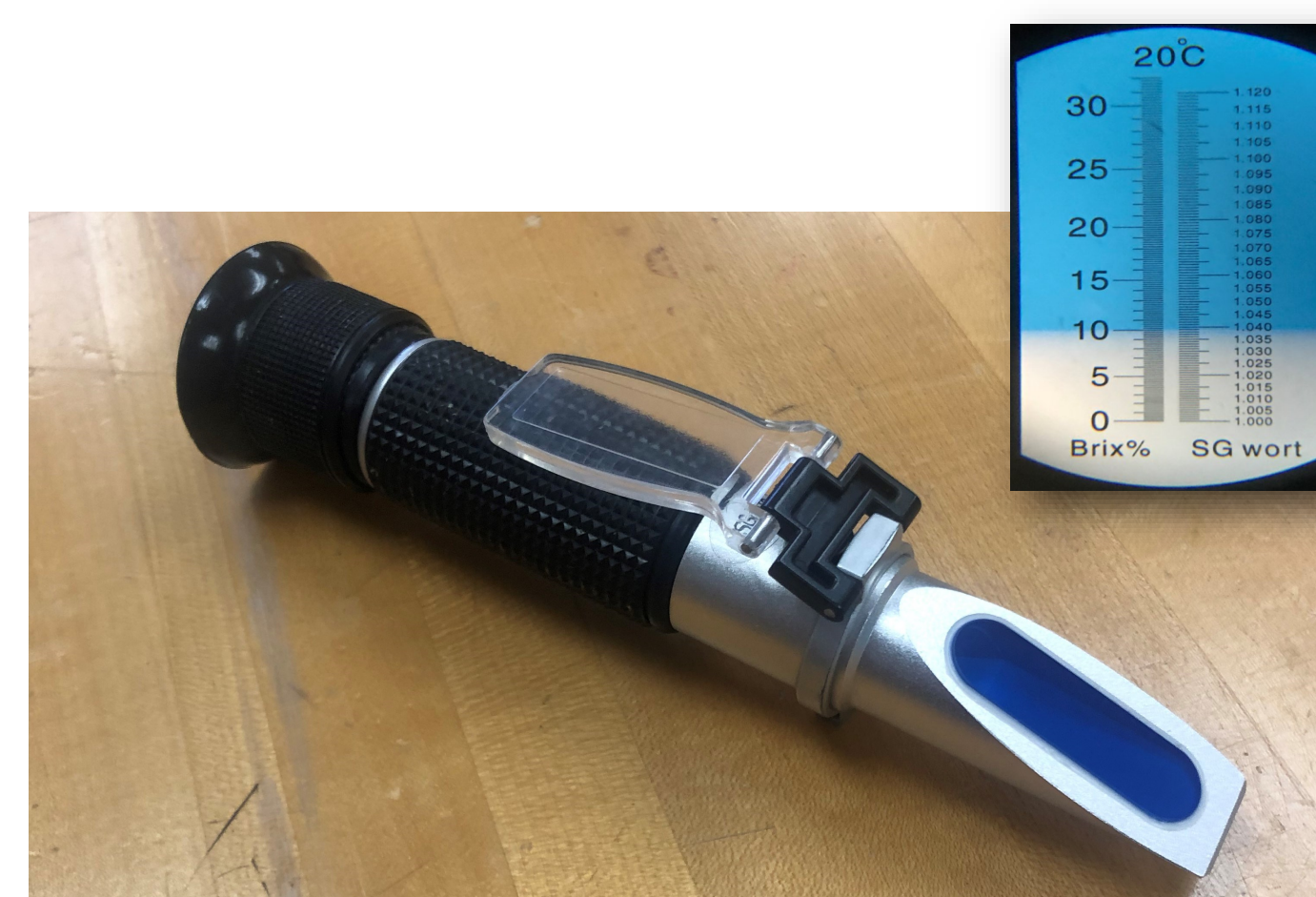
Figure 3. Brix Refractometer used to determine sweetness
