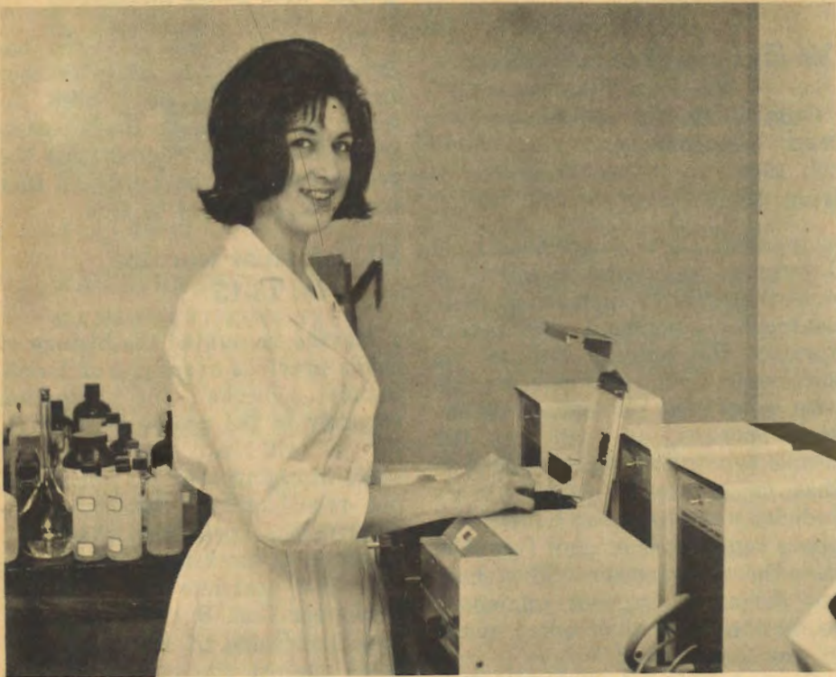
Myra Finch of the laboratory puts a tube in the Autoset, an electronic device which can measure the presence of barbituates in body fluids.
