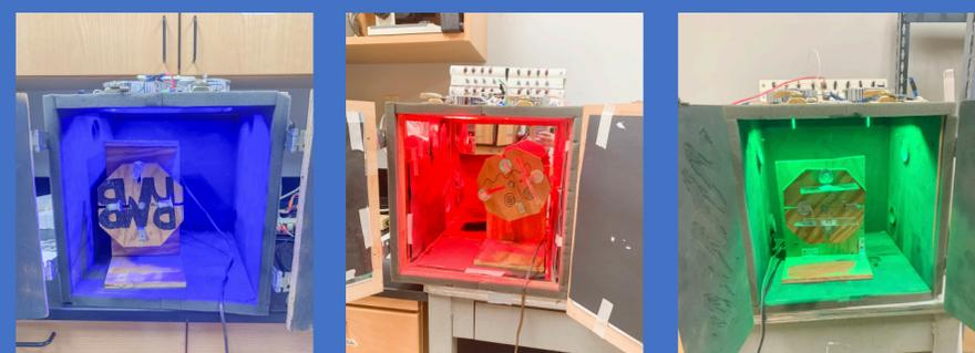
Figure 4: Blue- 460nm Incubator and clinostat. Figure 5: Red- 635nm Incubator and clinostat. Figure 6: Green- 525nm Incubator and clinostat.
