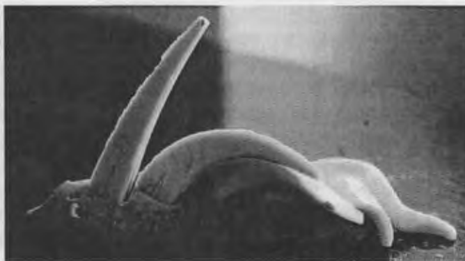
Fig.10. Pyrometric cones that have been fired to ^10
