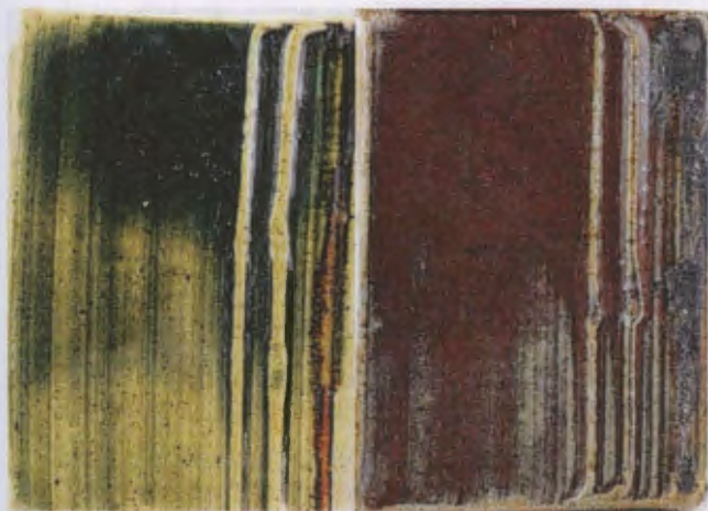
Fig.12. Meyers Clear with 3% added copper fired in oxidized, left tile, and reduced, right tile, atmospheres
