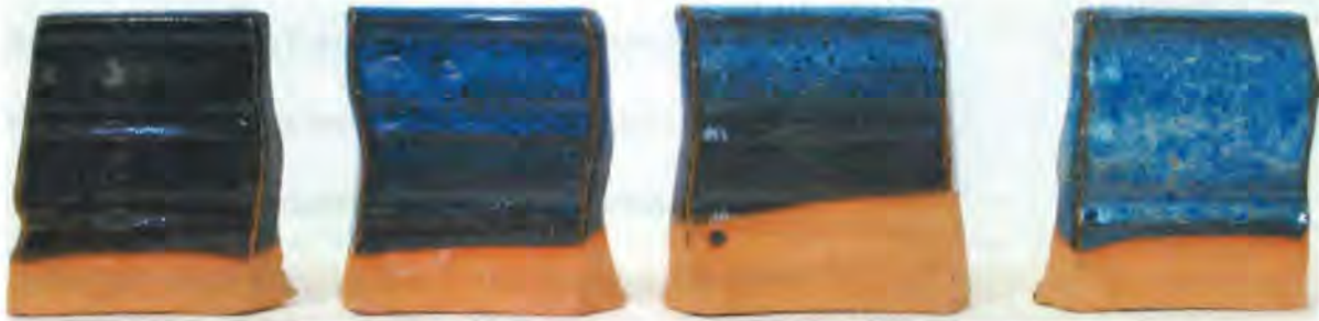
From left to right: 2% rutile, 2% rutile mixed with 4% rutile, 4% rutile, 4% rutile with thicker application
