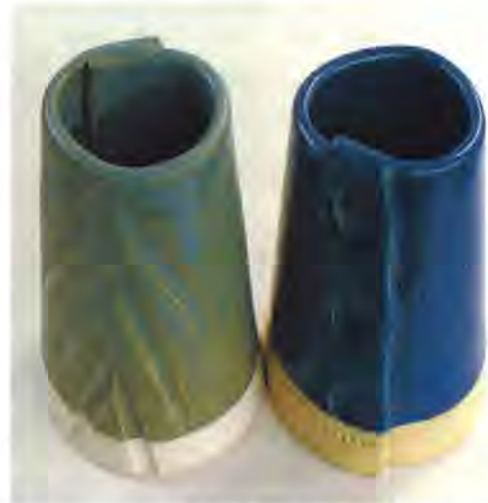
The same glaze in reduction (left) and oxidation (right) at cone 10. (Hansen, a)
