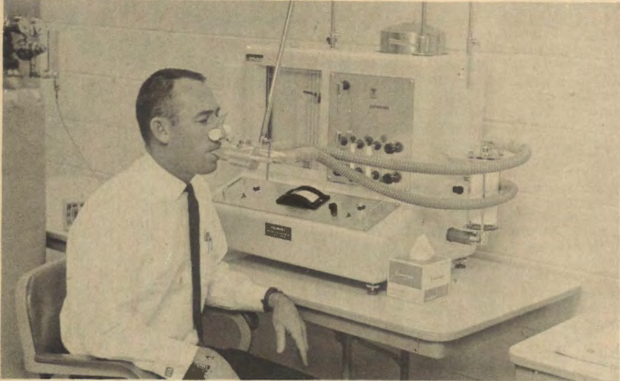
A company representative, Bill Stroman of Dallas, Tex., demonstrates how the patient breathes into the Pulmonet, one of the new pieces of equipment in the pulmonary laboratory for measuring lung volume.
