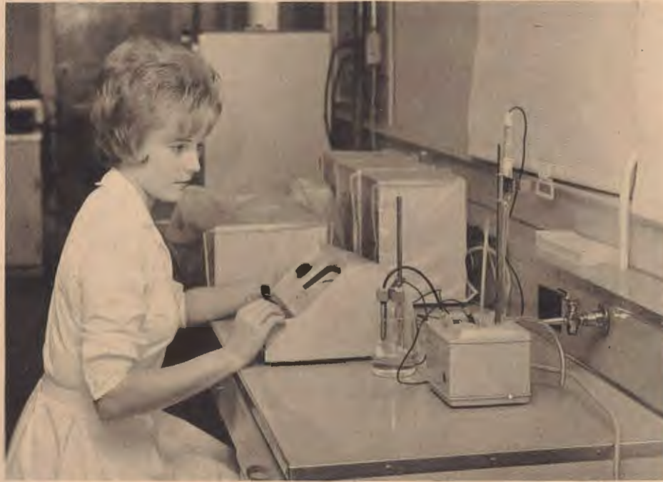
Louise Harris of the lab is shown with the Beckman expanded scale pH meter which can measure acidity or alkalinity giving doctors a clue as to what disease may be present.
