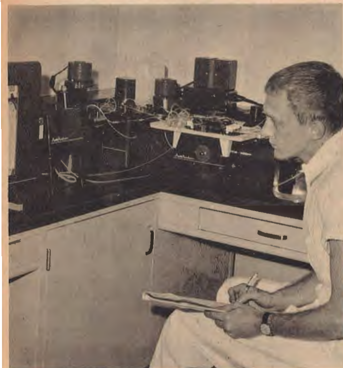
Bill Matthews, technician, records the readings on the autoanalyzer which a tiny sample of blood or other body fluid is run for analysis.
