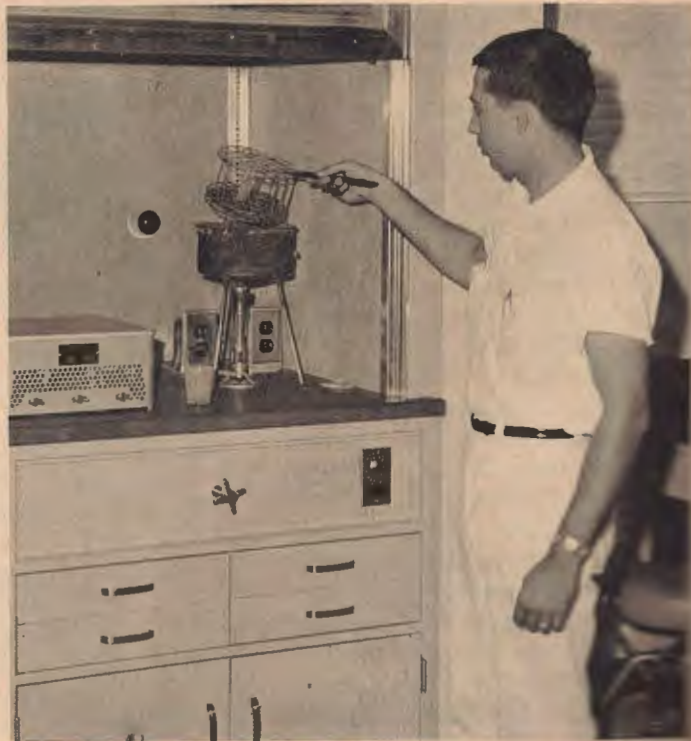
At right technician Aubrey Knight holds a test tube over a flame in the fume hood where gases and fume are carried off through a vent.
