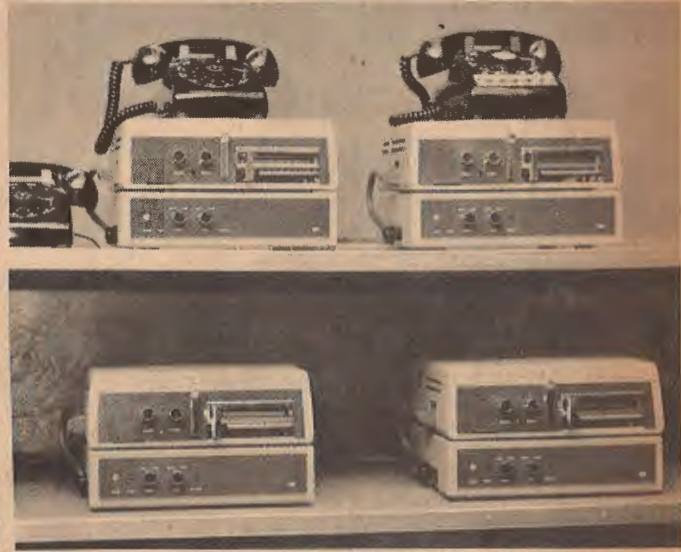
Dr. Julian Foster, at left, is dialing the number which will connect him with the dictating system, in the Medical Records Department. At right is the equipment which will record his telephone dictation automatically so that it can then be transcribed into typewritten records.
