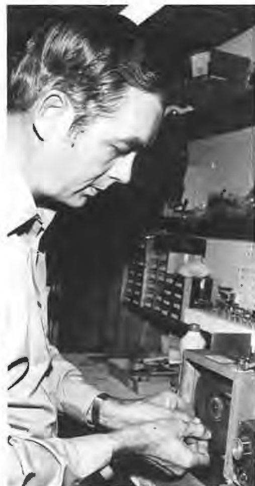
Lieutenant Colonel Kenneth Hestand, professor of military science, rounds the edges of a stone with a cabachon machine. Upon completion, the stone will be mounted on a piece of silver jewelry designed by LTC Hestand. The cabachon machine is similar to a saw only the blades are made of diamonds.
