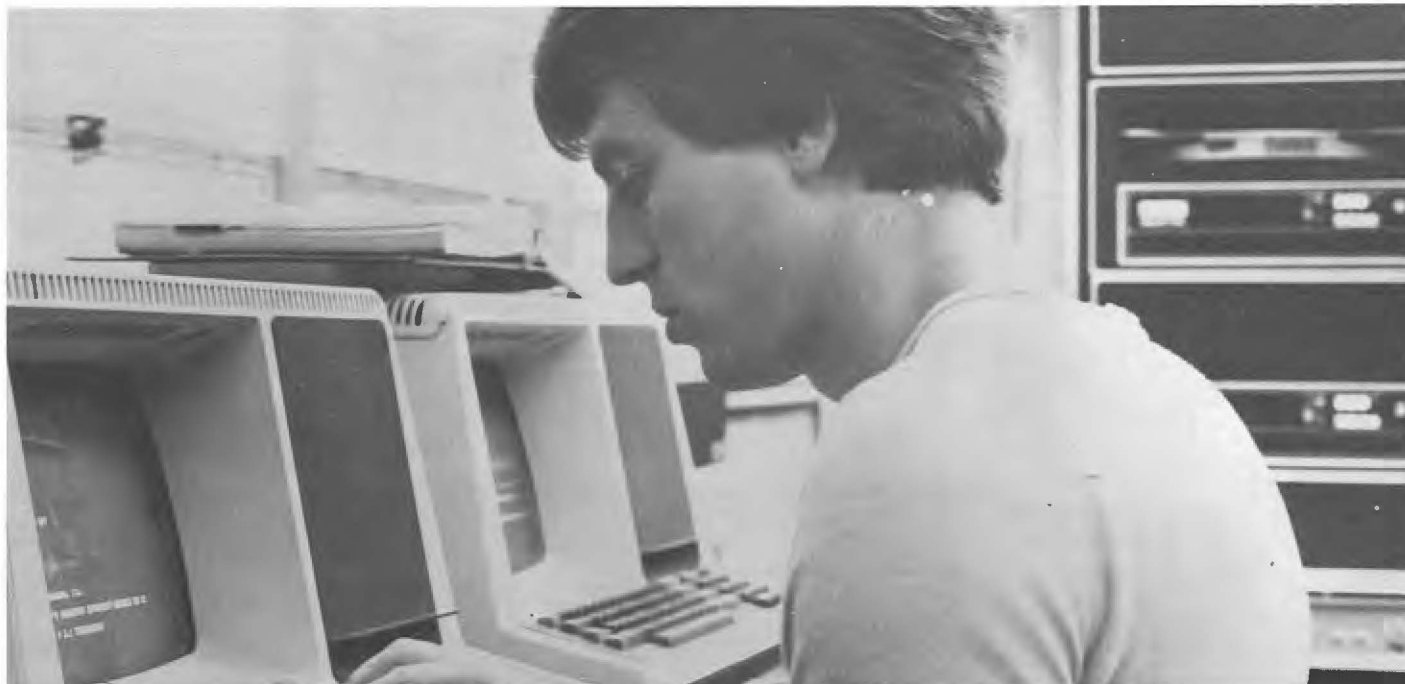
MULTI-PURPOSE COMPUTER —The new PDP-1134 digital computer in Moses-Provine Science Center is being used for teaching Fortran programming, calculating chemistry laboratory problems, tutoring, data handling in water research and other areas and will eventually be used to interface with other lab instruments, taking and processing data around the clock. Ron Burt of Mena, a '77 OBU grad and now a technician in water research, works on a program for Dr. Joe Nix.
